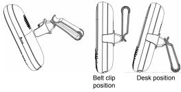
1. The belt clip/stand attaches to the back of the parent unit and clips into the locking slots on each side.
